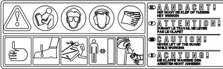
This sticker is affixed on the rear cover and warns the user not to open the cover while the machine is running. This sticker provides a summary of the general safety regulations by using icons: Art. no: BQ 505 010 360
