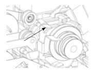
Next, remove the belt catchers from the belts by undoing the two bolts that hold the belt catchers.
