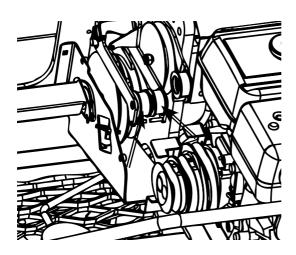
Due to belts being stretched during operation for a few hours, the manufacturer's settings can become disarrayed and the belts could begin slipping.
