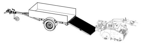
• If only two ramps are used, they must each have a width of at least 30 cm. The ramps put against each other for support of the central swivel caster provides a tread that corresponds to the width of the rollers.
