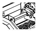
To remove the cover, undo the four bolts holding the cover in place.
