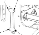
Demount the plate at the back of the belts after undoing the four M8 bolts.
