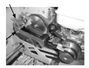
Unfasten the starlock locking clip at the back of the bolt. This will now have to be replaced also.
