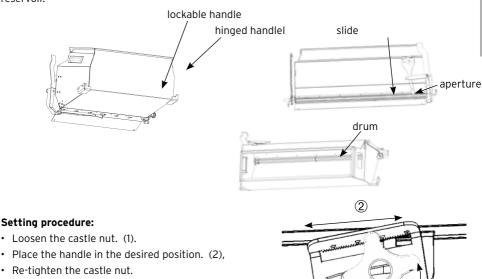
Placing the handle in a particular position determines the setting of the slide stop.
