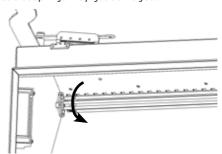
The position of the couplings can be corrected by manually turning the rotating drum in the seed reservoir.
