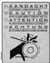
A safety sticker applied behind the large cover of the chain drive warns that no work must be done without the cover in place. Working without the cover poses the immediate risk of clothes or limbs getting caught in the drive and being cut off.
