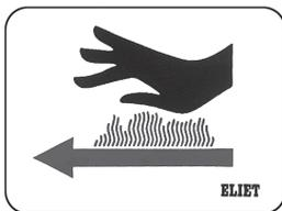
This sticker is affixed near the exhaust and warns the operator about hot surfaces with a high risk of burns.
