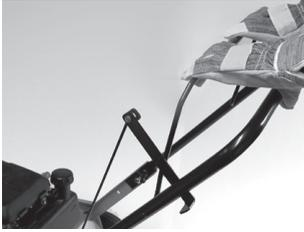
**Operation handle:** Releasing the operation handle disengages the blade drive from the engine, causing the blade axle to come to a stop.
