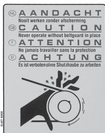
This sticker is affixed on the cover of the driving belt. It indicates the potential danger arising when the cover is removed while the engine is running. The machine may never be operated without the cover. The engine must be switched off before removing the cover at all times.
