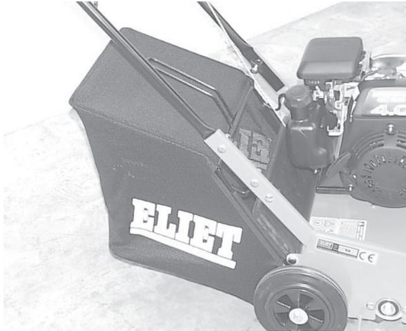
If the unit is full or the machine is losing moss, the unit must be emptied.
