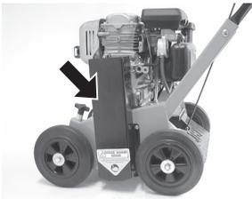
**Belt protection cover:** The cover ensures that all rotating parts of the driver that might cause injuries are adequately screened off.
