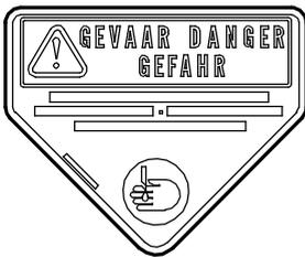
This sticker is affixed on the belt protection cover and warns about the danger of hand injuries. Keep your hands and feet away from underneath the machine as long as the blades are rotating. The engine must be turned off in case of faulty operation or before starting maintenance.
