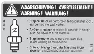
This sticker is affixed on the machine near the engine. The sticker reminds the user to switch off the engine and remove the spark plug cover before carrying out maintenance work on the machine.
