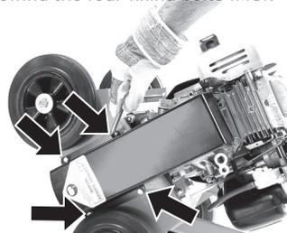
Provide support for the blade axle.
