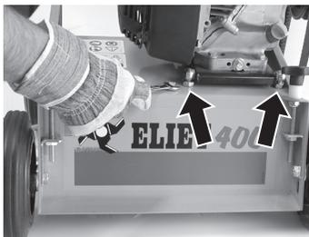
Tilt the scarifier by pushing the handlebar to the ground.
