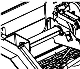
To remove the cover, undo the four bolts holding the cover in place.
