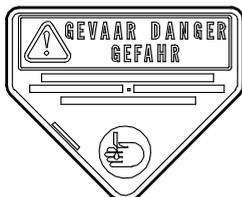
The sticker is located to the left of the frame, near the vibrating harrows. The sticker points at the danger of cuts when reaching hands or limbs into the relevant zone. This sticker carries stock code BQ 505 010 070.
