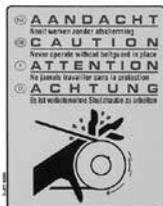
A safety sticker applied to the cover of the belt drive warns that no work must be done without the cover in place. Working without the cover poses the immediate risk of clothes or limbs getting caught in the drive and being cut off.
