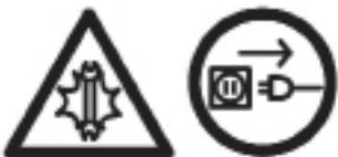
This icon ensures the operator will always disconnect the machine and will disconnect the electric plug from the machine as precautions when he or she wishes to perform maintenance on the blade system. This is to ensure that the machine cannot start up unexpectedly when the operator is performing maintenance with his or her hands near the blades.
