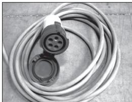
The direction of rotation of the blade shaft must be checked once the extension cord has been connected. If the direction of rotation is incorrect, reverse phases. (Read Annex 4.)
