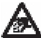
This icon warns of danger for kickback material. Chips are ejected from the discharge side of the machine at high speed. The collection box protects the operator and third parties against this projection. When the collection box is removed, this protection is also removed. This is the reason why we advise locking the collection box with the sliding latch to ensure that this cannot happen unintentionally.
