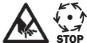
This icon points to the danger of cutting injuries to hands and ensures the user waits until the blades have stopped completely before opening the chipping chamber cover. Once the motor has been shut off, the blades will continue to turn for a short while due to inertia. This is a dangerous situation that we warn about here.
