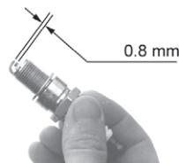
To verify the ignition quality, the following steps should be taken when the spark plug has been removed:
