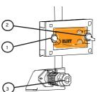
In order to disconnect the contact panel from the fixed tractor base, turn the star grip behind the panel, then slide it upwards over the rod. The plug is disconnected from the stand.
