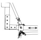
The height of the controls for the conveyor belt can be adjusted via the star grip. This is loosened and the rod can then be secured in the appropriate position.
