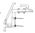
Fold the support base inwards so that the Eco Cure rests on the tractor.
