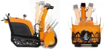
The same type of actuator is used to move the cutter head laterally 18° to the left or to the right.
