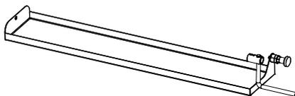
To adjust the seed flow rate, the stopper can be realigned. The position of the stopper determines the opening width of the seed outlets, and the amount of seed that will be spread.
