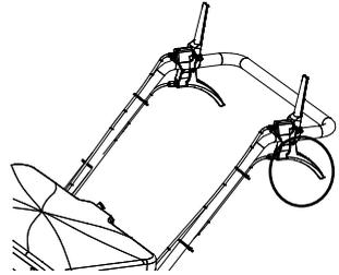
To change the machine from operating mode to transport mode, let go of the lever and push the steering gear down slightly.
