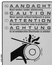
There is a safety sticker on the inside of the protective cover to warn against any work without the protective cover. There is an immediate danger of clothes or limbs being caught by the drive and cut off.
