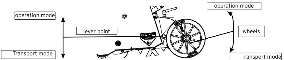
The lever on the left bottom side of the steering gear allows you to change the machine from transport mode to operating mode. To do so, the DZC's steering gear needs to be pushed down slightly, so that the pressure on the lock is removed. Then, push down the lever and lower the machine.
