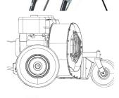
**Noise-reduced turbine:** a rubber-lined turbine wall provides considerable reduction of the noise levels, which is to the benefit of the operator's hearing.
