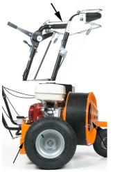
**Dead-man's handle:** This handle is mounted on the handlebar and must be pressed in order to start the engine. Releasing the handle disengages the engine.
