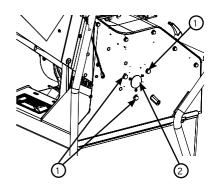
Now you can loosen the engine mounting plate from the frame. To do so, loosen the four M8 (3) bolts completely. The engine and its fixing plate are no longer attached to the chassis.
