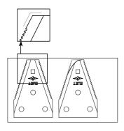
On the other hand, the form of the top of the blade is of essential importance for the performance and the speed of this primary chipping. The angle of the **top of the blade** will determine the angle at which the wood is pulled inside the shredding chamber. If this angle is rounded due to wear, the blades must be reversed and/or replaced. ("read § 11.3.6 Reversing and changing chipper blades" on page 43)
