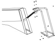
Place the handle in the feed hopper, align the upper holes. Insert a M6 bolt with flat washer true the feed hopper and handle.
