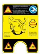
This decal is located on the protection chamber of the knife axle. It reminds the user to check the tension on the blade bolts regularly. The decal describes the manner of disassembly and assembly of the screen, and warns the user to switch of the engine before opening the screen.
