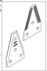
The position of the blades on the blade shaft has been selected very specifically to obtain an alternative chopping configuration with regard to primary chipping and the correct circulation of the chippings in the shredding chamber with regard to secondary chipping. You must, therefore, always ensure that you respect the original set-up when reversing or replacing blades. ("read § 11.3.6 Reversing and changing chipper blades" on page 43 where the rules are explained.)
