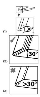
If the cutting angle is not maintained, blades will be stopped in the wood due to a blunt angle
