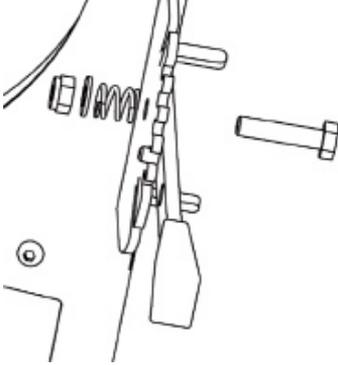
The rod that comes in the box connects the operation lever on the steering rack with the lever arm on which the blades are mounted. The rod is affixed to the lever on top via a star lock fastener. Underneath the rod, there is a screw thread to which the connection piece must be screwed. This is used for precision adjustments to depth. The axle pin on the connection piece is screwed into the hole in the lever arm and secured with a beta pin.
