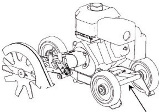
Turn the bar and secure it with the nuts supplied.
