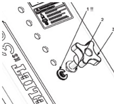
At the back, the rotational knob is secured with a nut.
