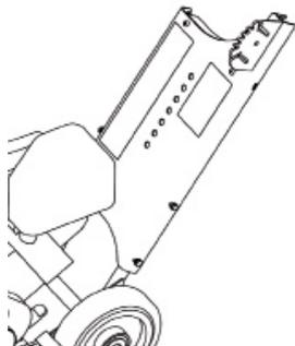
The second part of the bar is also assembled. This is done by inserting the bar behind the hook. This part is fully secured in the following step, when the rotational knob for height regulation is installed.
