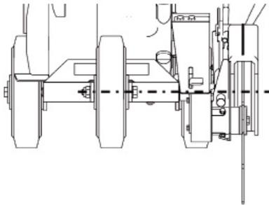
When tensioning the cord, ensure there is a safe distance between the wheel and the blade.
