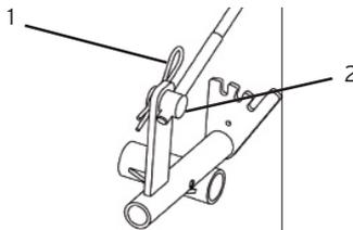
Pull the Beta pin (1) out and take the screw (2) out of the holder.
