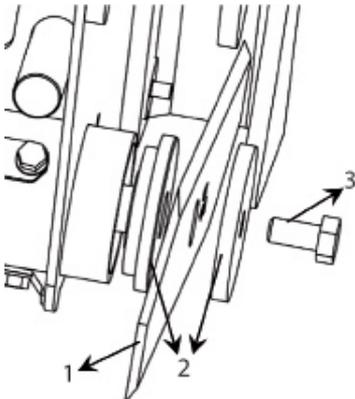
When removing the blade, note the order of the machine parts that have been removed; this will simplify reassembly.
