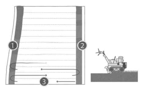
In doing so two deeper zones are created at the extremities of the work zone. After turning it will be easier to get the blade to work depth when beginning the new strip. This allows you to work faster.
