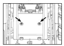
• Use a lubrication pump to slowly pump extra lubrication grease into the bushings. Use the lubricant shown in the list in "11.3. Lubricants" on page 62.
