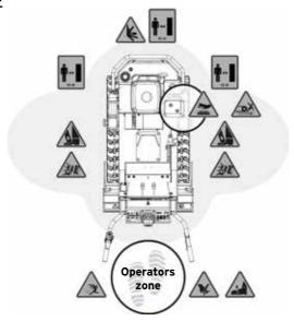
• The operators zone is situated behind machine with both hands on the handlebar. This is where there is best access to the operating elements giving control over the machine.
