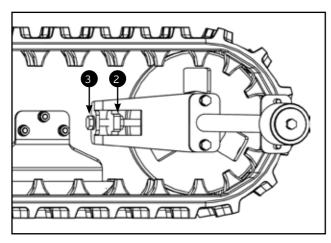
Now screw the locking bolt M10 further in (clockwise) so that the back shaft is pressed backwards and the track becomes tense. (ring wrench size 17). Do this on each side of the machine until the correct tension is achieved.
