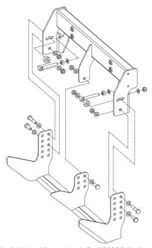
Before tightening the blade, set the correct angle. Read "§ 9.2.3 Setting the angle of approach" on page 32.
