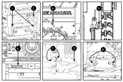
On these friction surfaces you must ensure there is lubricant between the rubbing parts in order to reduce the resistance on the movement and prevent the elements wearing.
