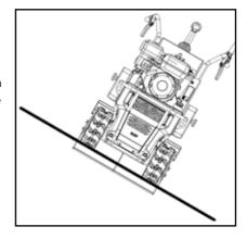
(Place the machine with the left flank on the side of the valley in order to start up again). The solution is to wait a few moments before restarting the engine on a level surface. The problem will reoccur if you continue to do work on a slope. After checking the oil level on an even surface (read § 11.4.3; page 64), the oil safety system may be disengaged temporarily. Do not forget to switch it back on afterwards.
