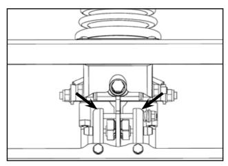
The level of operating stiffness can be adjusted by adapting the pressure of the brake pads on the friction plate.
