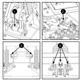
If slack is perceived at these points the machine must be taken to the ELIET dealer for repair.
