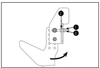
• If the aim is to reduce the angle of approach it is necessary to twist the nut on the inside of the holder in a clockwise direction (1) so that this comes loose from the holder. Then, turn the nut on the back of the holder with a size 17 ratchet in a clockwise direction (2). This causes the blade to stand straighter, thus decreasing the angle of approach. Once the required angle is set, the nut on the inside must be firmly re-tightened, to sit tight against the holder. (3).
