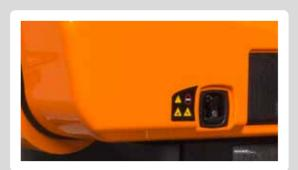
The large, tightly formed protective covers have just one subtly integrated closure. This special **grip** ensures that the cover is securely attached to the frame to **prevent disruptive vibrations** during operation or transport. The grip is fitted with a lock to keep the engine and drive technology safe and secure.
