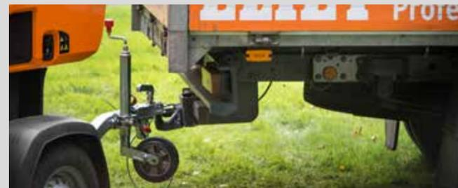
The chassis is a sturdy, fully welded and galvanized frame. This rigid frame rests on a spring-loaded axle with a wheelbase of 180 cm. In combination with a low center of gravity, this provides excellent road holding. The trailer is fitted with a height-adjustable support wheel and two extendable support legs that enable stable setup once unhitched. It comes standard with chocks.
